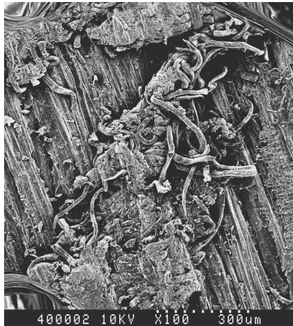
FIG. 1. Scanning electron microscopy image of entangled beech wood fibers in a matrix of melted intercellular material obtained by linear flat welding of wood.
