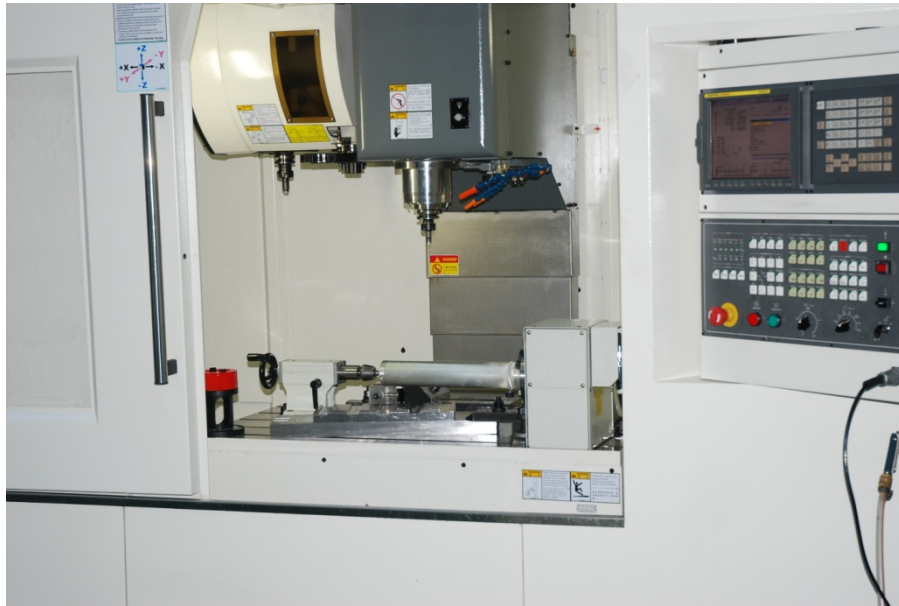
Fig. 5. The workpiece prepared for friction welding on the adapted numerically controlled milling machine
