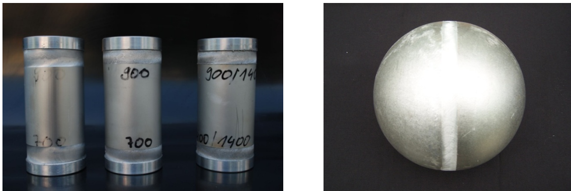
Fig.4. Examples of fabrications friction welded using the new technology. a) pipes welded with covers; b) valve balls
