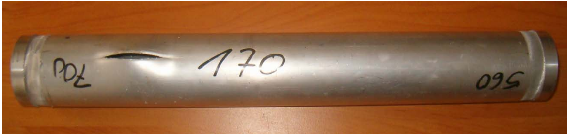
Fig. 6. The pipe was destructed at the pressure of 17 MPa without damaging the welds
