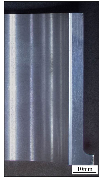
Fig.10 Cross section of coated cylinder with 80mm diameter
