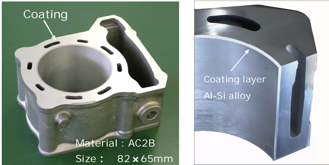
Fig.16 Cross sections of coated aluminum cast engine block
